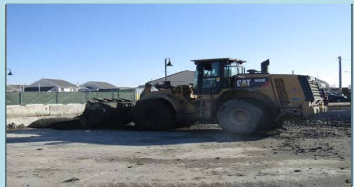
6 Cat 966 loader moving material to the North Pad for staging
