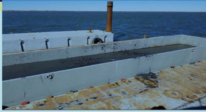
1 Loaded scow ready for dewatering
