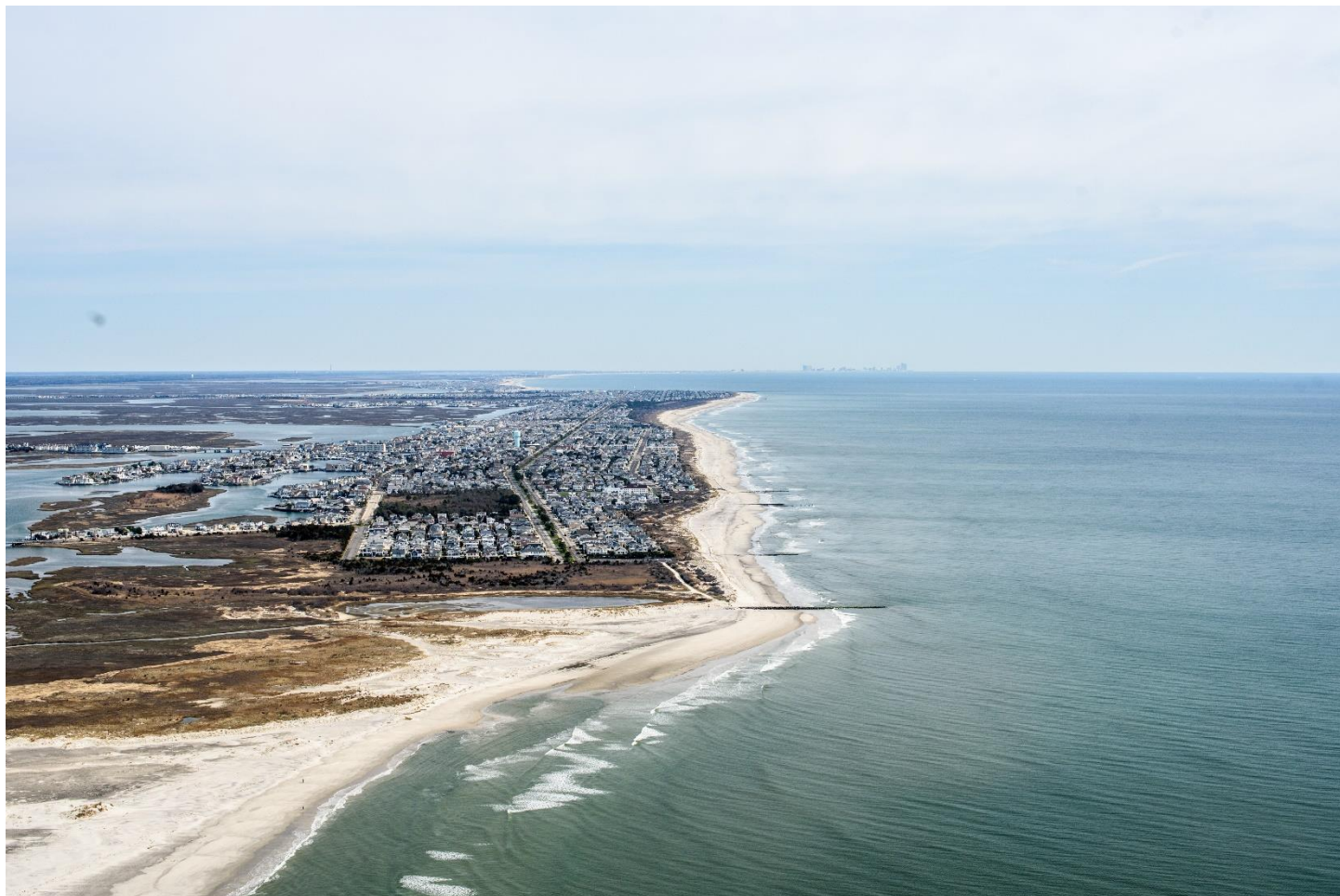
Aerial photograph taken April 21, 2018 showing the view up the beach from Stone Harbor Point beach. Note the new deposit of sand extending south from the terminal groin. This is sand derived from the 2 nd Periodic Nourishment Cycle in the Borough's southern section moved beyond the groin by the series of northeast storms in March/April (courtesy Ted Kingston).
